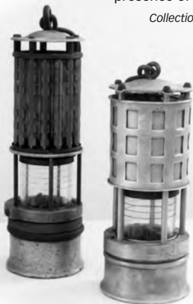
Below: Flame safety lamps (left, 1935; right, 1950) tested mine air for oxygen levels and the presence of methane gas.
