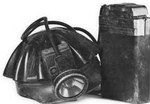
Above: A miner’s hard hat with electric lamp and battery, early twentieth century
